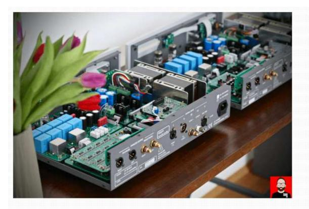
To observe real differences, lids would need to be popped. Sitting the open Optologic box next to its predecessor, we see how the Formula's four separate ladder DAC boards, populated with "low noise precision resistors", have been distilled into a single slab that sits top right as we observe the Optologic DAC from front to back.
