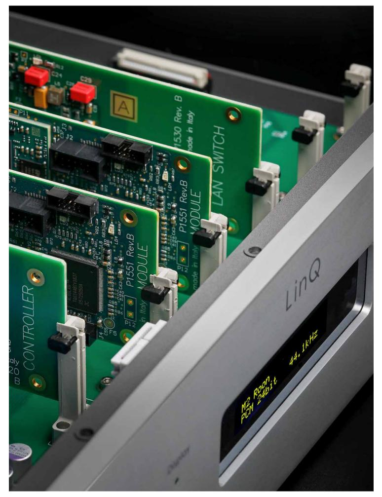
Modular design principle: Aqua incorporates all of the LinQ's important functions into plug-in cards—UPnP streaming, Roon access and so on. This ensures that virtually any future upgrades and subsequent additional functions can be incorporated into the network bridge.
