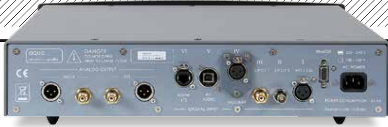
ABOVE: Six digital inputs are offered including S/PDIF (RCA and BNC), AES/EBU (XLR), USB-B for computer connection, I 2 S 'AQlink' (RJ45) and a module option for one more of the same (also Toslink optical). Fixed analogue outs are offered on single-ended (RCA) and balanced (transformer-coupled XLR) connections
