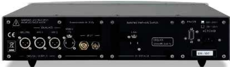
ABOVE: Aqua offers a single wired Ethernet port by way of input, feeding single and dual-AES/EBU outputs on XLRs, S/PDIF outputs on coaxial and BNC connectors, and an I S output via an RJ45 connection (this is not a network port)
