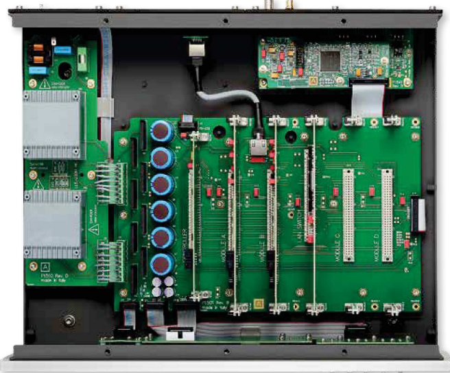
RIGHT: Two transformers [near left] feed separately regulated PSUs [blue caps] that supply the custom LAN switch card [far right], Roon and UPnP/DLNA cards [centre] and digital decoder [on an Altera FPGA, top right PCB]
