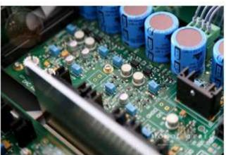
Aqua implanted passive components to achieve reliability, longevity and best sonic quality. With the exception of six superior electrolytic capacitors, all other caps are Tantalum, solid-polymer OS-CON and double-metalized MKPs. The signal path itself is direct-coupled and in complete absence from the capacitors.
