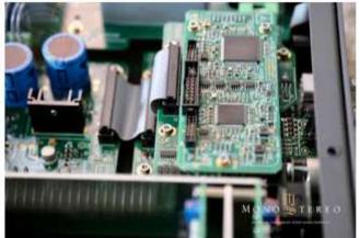
The Formula has a sign-magnitude converter structure, and this requires not two but four 24 bit resistors banks, each one made of very low tolerance discrete resistors. In order to separate the digital section from the sensitive analog circuits, galvanic and magnetic isolations are implemented between the FPGA and the four branches of the R2R ladder converter.
